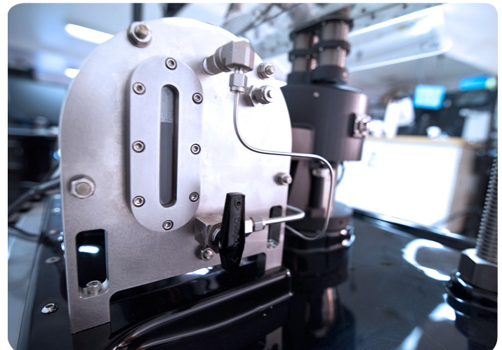
High-pressure capacitance tank with observation window and float switch.
