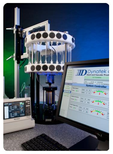
Dynatek Labs performs radial pulsatile durability and fatigue testing, and bend testing of vascular stents and stent grafts compliant with the following standards:
