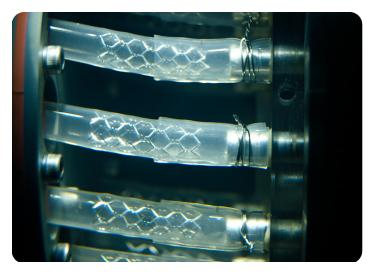
Dynatek Labs performs radial pulsatile durability and fatigue testing, and bend testing of vascular stents and stent grafts compliant with the following standards:
