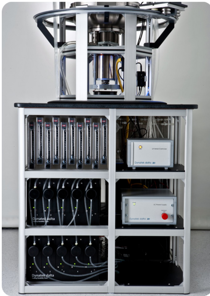
Lower section of the CDT-20 showing flow meters, controller, and particle counters.
