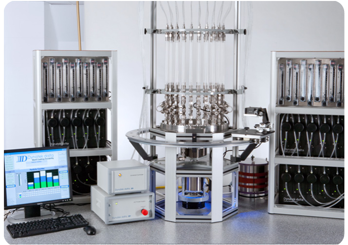
Dynatek's CDT-20 benchtop Coating Durability Tester
