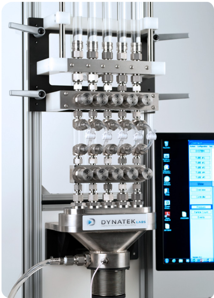
Five stent samples in straight, curved or bifurcated mock vessels
