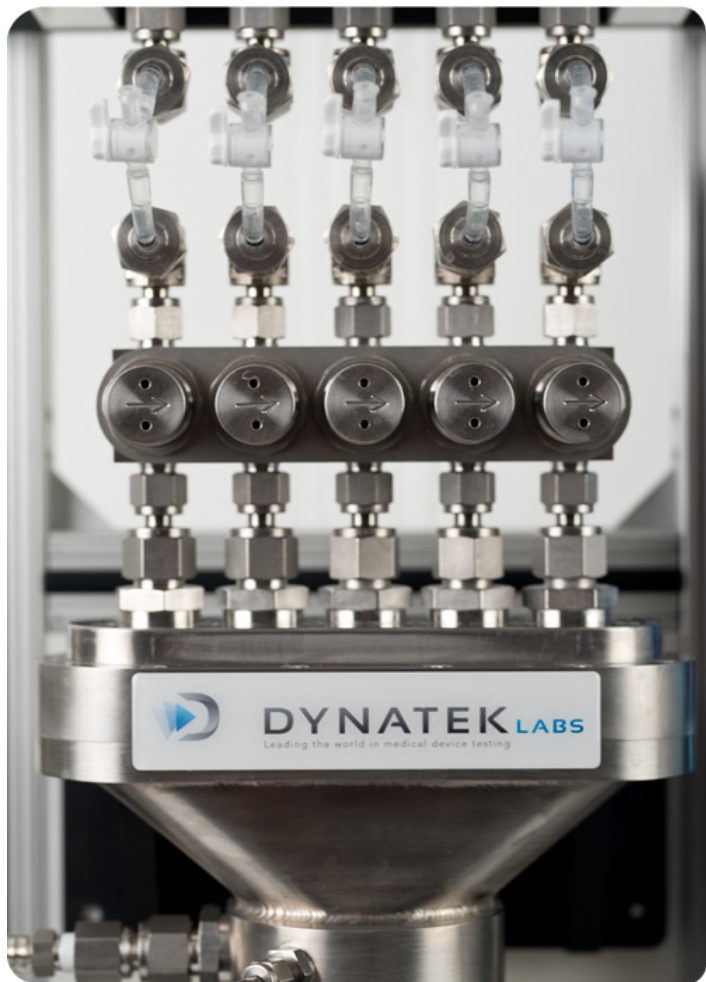
Shut-offs for each sample makes individual removal easy
