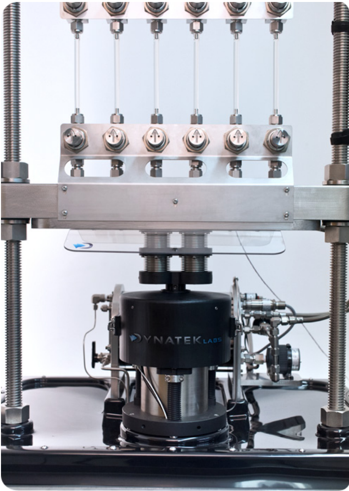
The FtF tester supports up to six samples.
