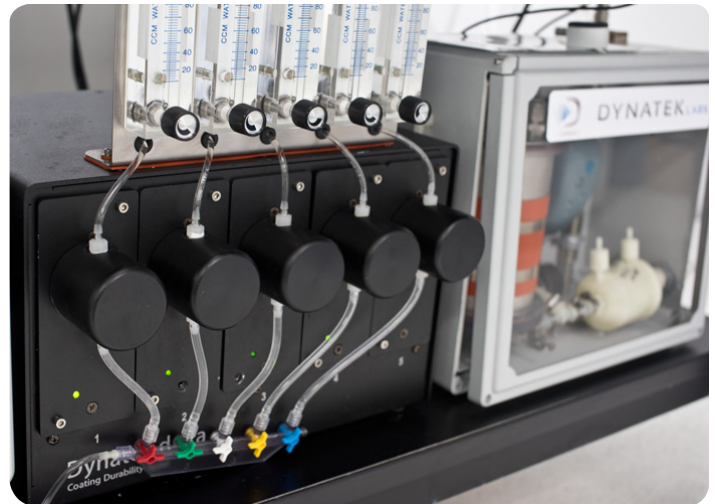
Flow control, variable pump, adjustable heating, inline filter.
