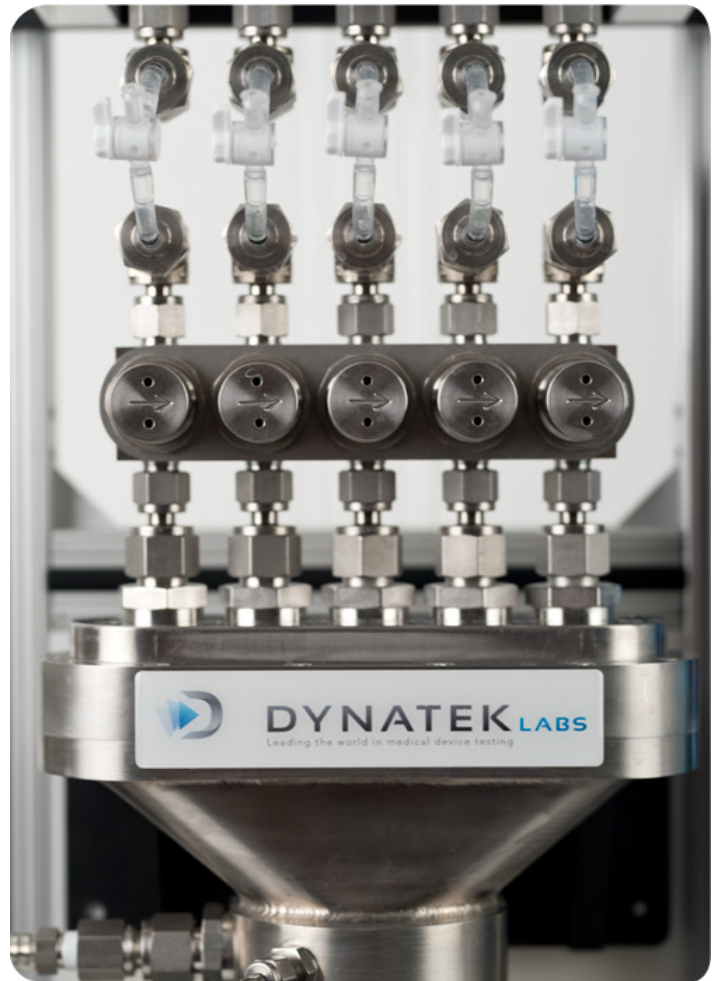
Shut-offs for each sample makes individual removal easy
