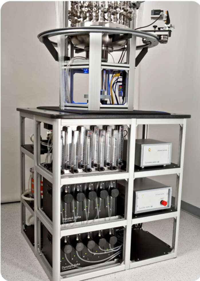
Fig. 3: CDT-20 Coating Durability Tester, using 4 particle counters (2 located in the front, 2 located in the back) for a total of 20 sensors, one for each sample.
