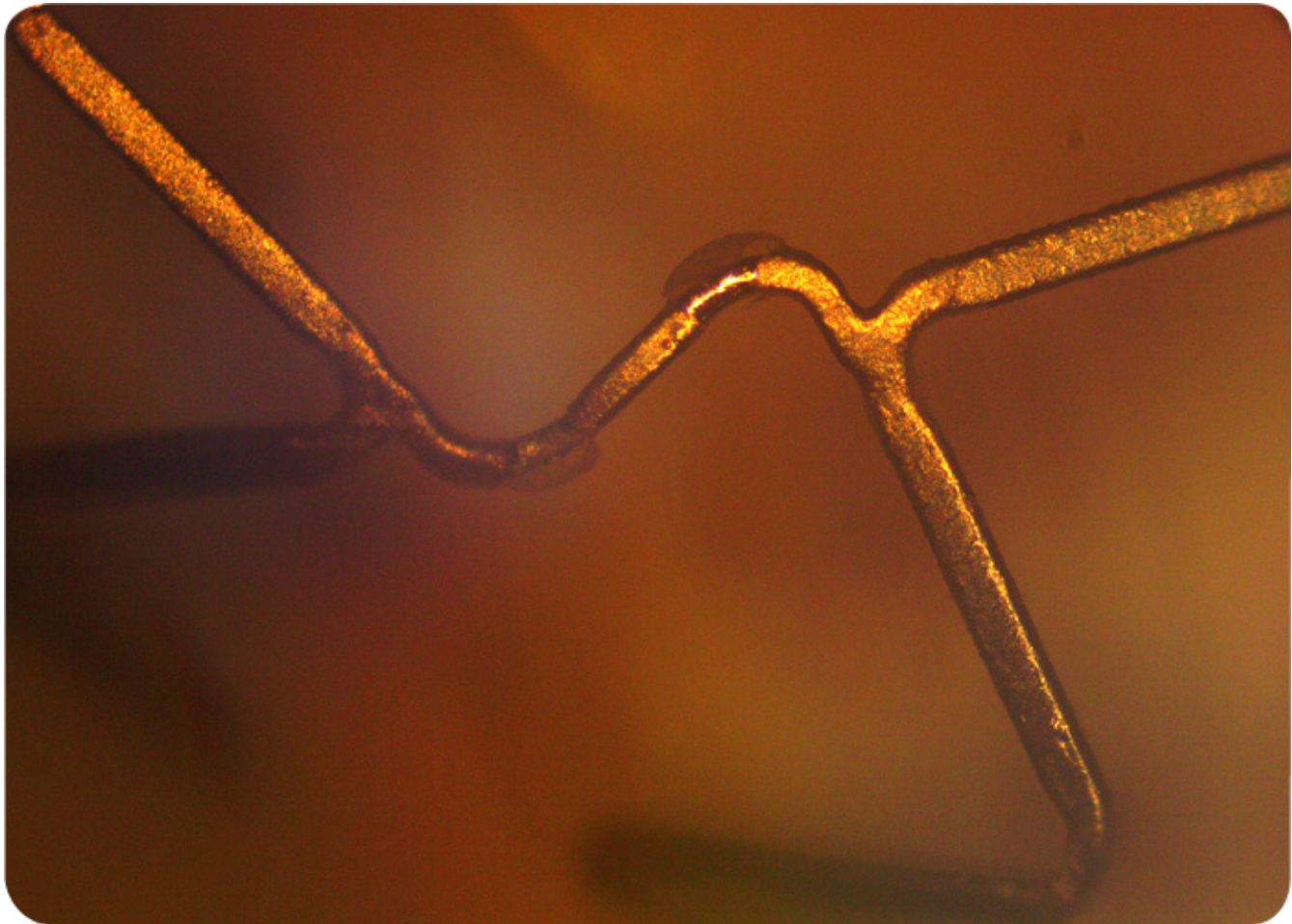
Fig. 1. Blistering of stent coating, 40x
