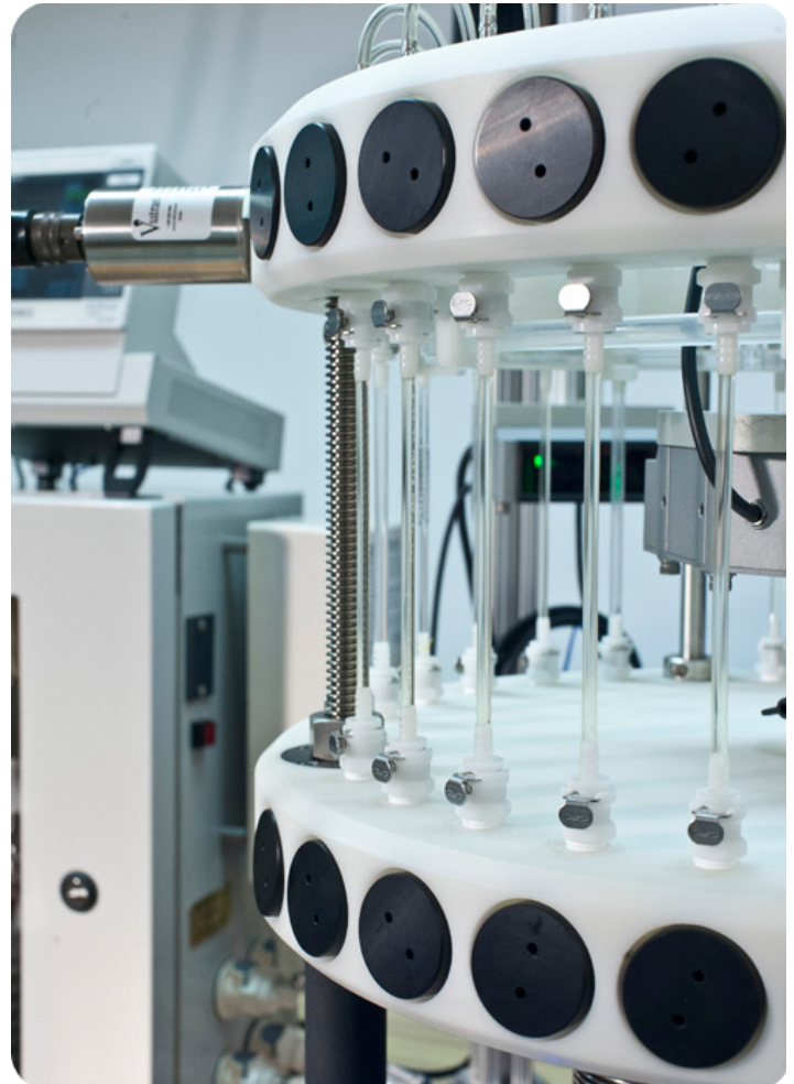
Fig 3: UST stent tester, showing laser micrometer focused on sample
